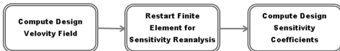
Fig. 27.2 Design sensitivity analysis process
