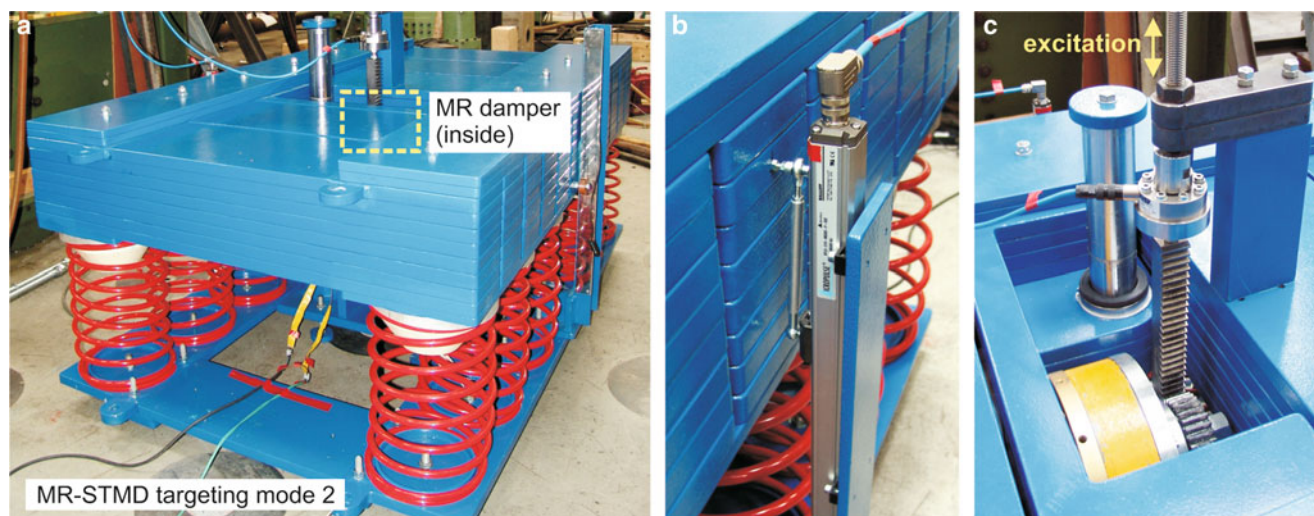
Fig. 10.7 Single full-scale MR-STMD: general view (a), displacement sensor (b), MR damper installation and force sensor (c)
